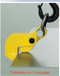
The THK horizontal plate clamps share the same basic design features as the CH range of clamps but have a reversed tooth jaw design. This safety feature is designed for use with thin sheets which may have a tendency to deflect or sag or flex.
