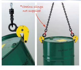
The DC500 drum clamp has been designed to lift and transport steel drums. If moving empty or sealed drums then one clamp is sufficient. Should you be lifting an open full drum, then two clamps should be used with a two leg chain sling.
