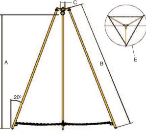
The Camlok Shearlegs have been designed to be simple and easy to erect and operate. Each set of shearlegs are supplied, as standard, fitted with safety chains and a large eyebolt for the suspension of hand operated lifting mechanisms, chain blocks or pulleys.
